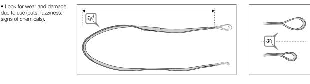
• Check the condition of all safety stitching on both sides. Look for any threads that are loose, worn, or cut.
