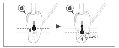
• Verify that the attachment point opens when the opening lever is pushed to the right. Verify that the lever returns to position when released.
