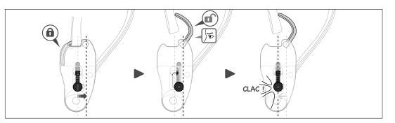
• In case of dirt impeding the function of the lever, clean with soapy water and lubricate in the three places indicated in the diagram.
