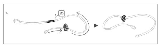
• Reinstall the strap on the pulley.
