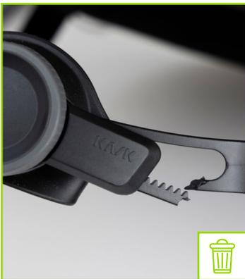
Broken adjustment system branch
