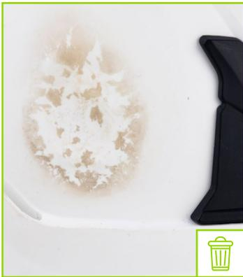
External shell with traces of chemical substance
